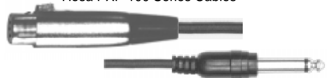
Figure 6a. For signals coming into the bay from balanced equipment that features XLR outputs, use a cable like Hosa's PXF-100 series, which "unbalances" the signal (ground "shares" the negative conductor) for use with the PHB-265 when using the half-normalled or full-normalled configurations.
